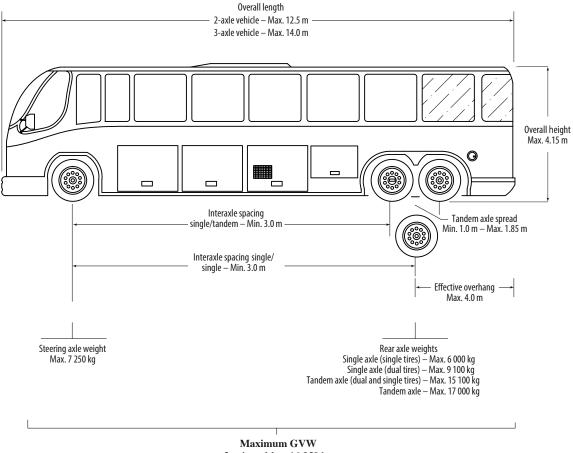
2 axles – Max. 16 350 kg 3 axles – Max. 24 250 kg
