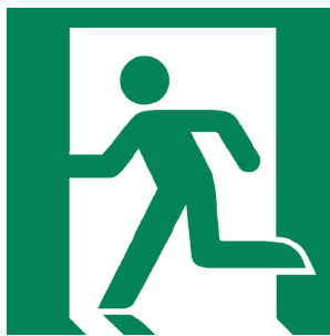
Figure A-3.4.5.1.(2)(c)-A “E001 Emergency exit (left hand)” (E001) symbol from ISO 7010
