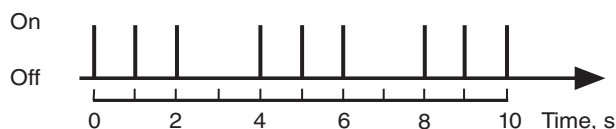
Figure A-3.2.4.18.(2)-B Temporal pattern imposed on a single stroke bell or chime
