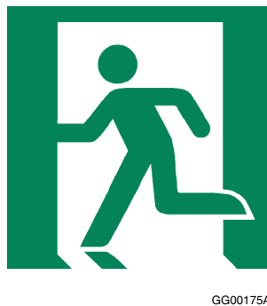
Figure A-3.4.5.1.(2)(c)-A “E001 Emergency exit (left hand)” (E001) symbol from ISO 7010
